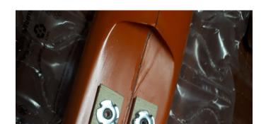
Glue the wood and the nuts inside the fuselage with epoxy
