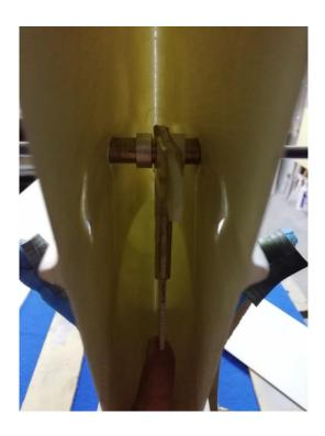
INSIDE THE TAILPLANE THERE IS A MAGNET ABLE TO JOIN IT TO THE STEEL BAR
