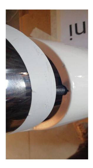
Make a slot in the front side of the fuse
