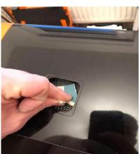
Sand the gluing surface
