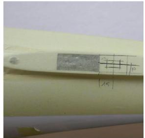
Open the windows (with Dremel blade) – we use MULTIPLEX GREEN CONNECTOR (MPX 6 pins – female).
